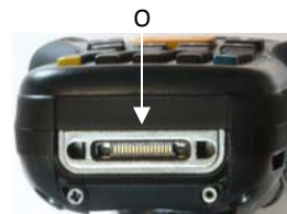
O) Handylink connector (host/client)
